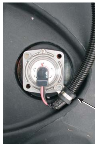
Clamp the harness at the gauge, seal the split sleeving with silicone sealant.
