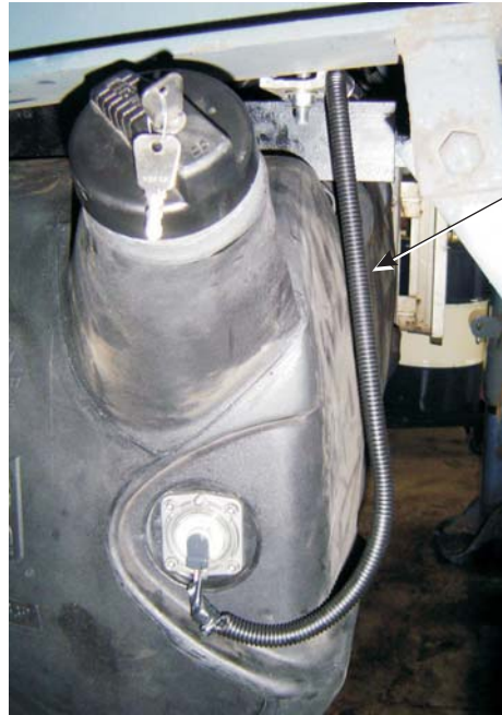
Use split sleeving to protect the harness
